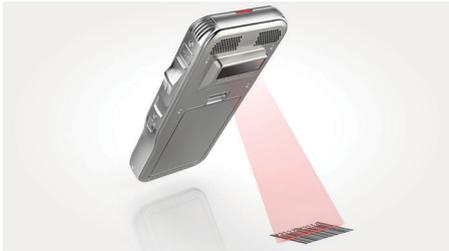
The integrated barcode scanner enables you to link client or patient data to a recording by simply scanning over a barcode, even from a display.\* This ensures reliable assignment of client or patient IDs and speeds up your workflow.
