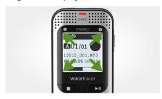
The large backlit display allows you to see all important file information clearly at a glance. This makes file navigation easier, even in low-light situations.
