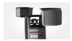
The metal grille comes with specially designed hexagonal openings which allow three times more sound to reach the microphone than its predecessor, engineered to provide crystal clear recordings. A fleece inserted above and below the microphone capsule filters out sound distortions such as pop and hiss noise, guaranteeing perfect results even if dictating closely into the microphone.
